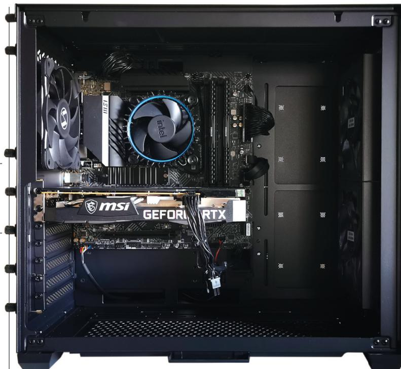
The 650W PSU offers bags of spare capacity: the PC draws 49W at idle with a peak of 300W. So, how to take advantage of those extra watts? The MSI board offers a couple of upgrade routes, with two PCI-E slots lying empty (one x16 and the other x1), along with one empty spare M.2 slot. This supports Gen 4 drives, as does the main slot, but the supplied 500GB MSI drive is Gen 3, with fast sequential read and writes of around 2,800MB/sec.
