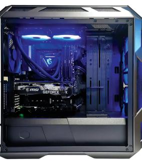
ABOVE The glass panel on the front can be swapped for a metal mesh
