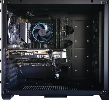
The 650W PSU offers bags of spare capacity: the PC draws 49W at idle with a peak of 300W. So, how to take advantage of those extra watts? The MSI board offers a couple of upgrade routes, with two PCI-E slots lying empty (one x16 and the other x1), along with one empty spare M.2 slot. This supports Gen 4 drives, as does the main slot, but the supplied 500GB MSI drive is Gen 3, with fast sequential read and writes of around 2,800MB/sec.
