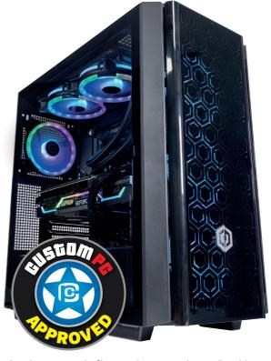
has done a great job of keeping the interior tidy as well, and the main areas of the build are accessible. The chassis supports 360mm radiators as well, and it can accept another hard disk and two 2.5in drives, but it also misses some finesse – it has no tool-free storage bays, no USB Type–C connector and no button to alter the lighting.
