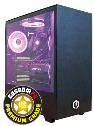
All this gear is housed in an NZXT H511 chassis, which is a modified version of the common H510, although disappointingly, it lacks a USB Type-C port. Elsewhere, build quality is solid and it looks smart, with a sleek front panel, clean lines and a tempered glass side panel. The 210mm width and 460mm height make it relatively compact too.
